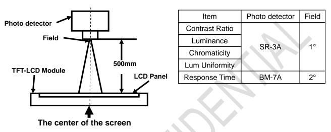
Note 2: Definition of viewing angle range and measurement system.
