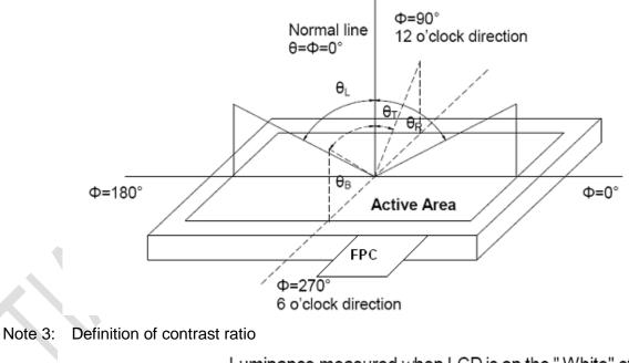
Contrast ratio (CR) =  $\frac{\text{Luminance measured when LCD is on the "White" state}}{\text{Luminance measured when LCD is on the "Black" state}}$
